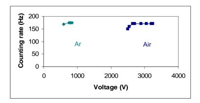
Fig.7. Counting rates vs. the applied voltage measured in Ar and in air under the same conditions (alpha particles, D=60mm, da=100  $\mu$ m)
