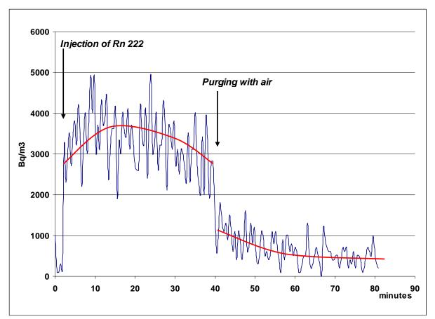
Fig.15. Counting rate vs. time after injection into the basic design (at t=2min) of air contaminated with <sup>222</sup>Rn. At t=40 min the detector for a few second was flushed with clean air
