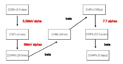
Fig.18. Chain of <sup>222</sup>Rn decays. Our single-wire counters were mostly sensitive to alpha particles emissions
