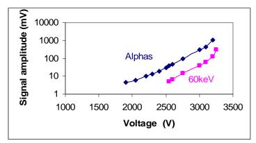
Fig. 6. The pulse amplitudes vs. the voltage measures with a single-wire counter having D=30mm and  $d_a=100\mu m$ . One can see that at  $V_d>3250V$  the pulse amplitudes start deviating from the strait line in the log scale indicating the appearance of feedback processes. This effect was not observed in the case of detector having D=60mm and da=100 or 25  $\mu m$
