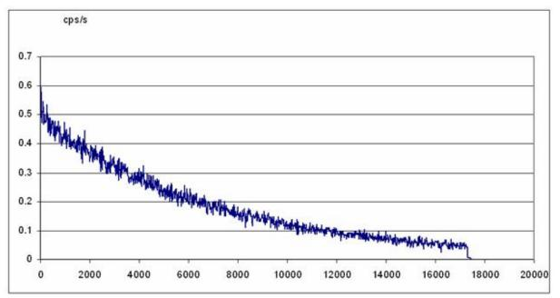
Fig. 17. Long-term measurement performed with the ionization chamber: the counting rate decrease with a good accuracy corresponds to the decay of the  $^{222}$ Rn (T<sub>0</sub>=5500min)
