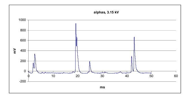
Fig.9 . Pulses produced by a <sup>241</sup>Am in 100% humid air
