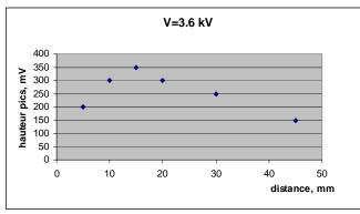
Fig. 25. Alpha particles signal amplitude as a function of the distance from the single-wire counter
