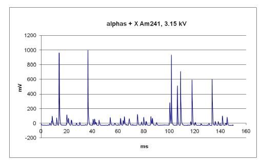
Fig. 4. Typical signals observed with the single–wire counter (basic lay-out) working in air and irradiated with a  $^{241}$ Am source
