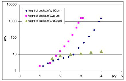
Fig 5. Mean signal amplitude produced by alpha particles vs. high voltage in a detector with cathode diameter of 60 mm and varying the anode diameter
