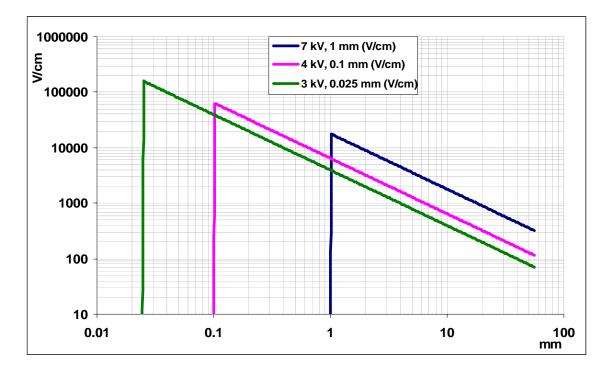
Fig.1. Electric field in a single wire counter as a function of the distance from the anode wire diameter:  $25\mu m$  (green),  $100 \ \mu m$  (rose) and  $1000 \ \mu m$  (blue).
