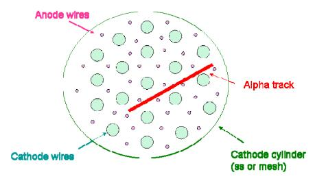
Fig.3. Schematic cross section of the MWPC sensor.
