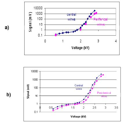
Fig 19. MWPC gain vs. voltage measured with alpha particles oriented perpendicular to anode wires(a) and parallel to them (b)
