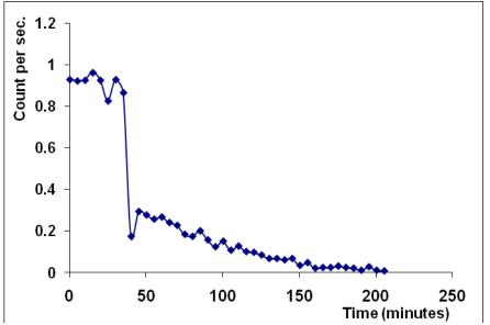
Fig. 16. Counting rate vs. time when the radon contaminated air was introduces (at t=0 sec) into the ionization chamber and at t=40 sec it was flushed with clean air. The fast decrease of the counting rate is mainly due to the Po decay
