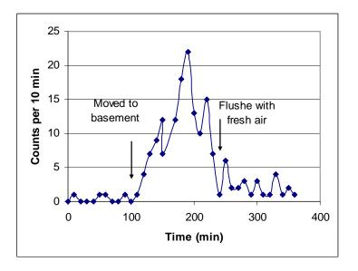
Fig.23. Performance for a small concentration of Rn in a basement. In the time interval of 0-100min, the MWPC has been operated in fresh air. At t=100min, it was moved in to the basement. At t=240min the chamber was flushed with fresh air and removed from the basement
