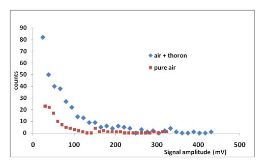
Fig. 14. Pulse height spectrum of Thoron and noise induced pulses
