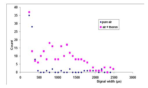
Fig.13. Distribution of the width of noise and Thoron induced pulses
