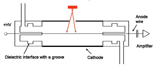
Fig.2. Schematic drawing of the single-wire counter working in humid air at high gain.
