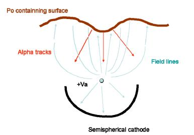
Fig.24. A schematic drawing of a single-wire counter for the monitoring of the presence of Po.
