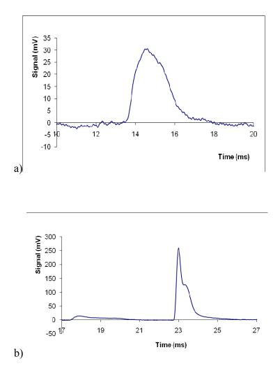
Fig.11.Typical shape of pulses produced in the single-wire counter by Thorium: a) smooth pulses, b) pulses containing 1-2 peaks
