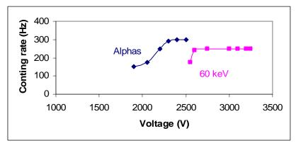
Fig.8. Counting rate vs.  $V_d$  for alpha particle (blue) and for 60 keV photons (pink) measured with a basic design of the single-wire counter
