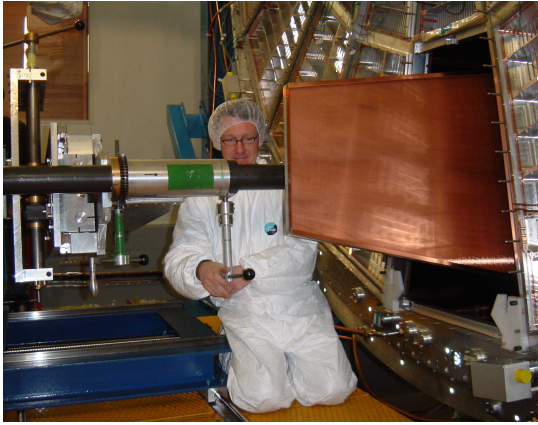
Figure 17: Insertion of an OROC through the endplate. The tilt, polar and azimuthal angles of the chambers can be adjusted via handles and a transmission system.
