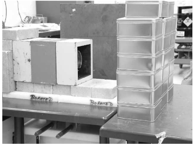
Fig. 5. Experimental setup to measure the decay spectra of different isotopes (see text). On the left hand side the germanium spectrometer covered by a lead shielding is shown. The radioactive isotopes were placed into the gap between the spectrometer and the metal boxes on the left.
