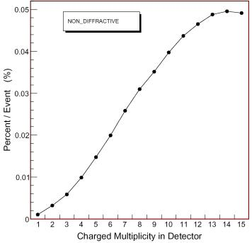
**Figure 7.** The efficiency to detect non-diffractive events (ND) by the Forward Shower Counters (FSCs) as a function of the charged multiplicity in the detector.
