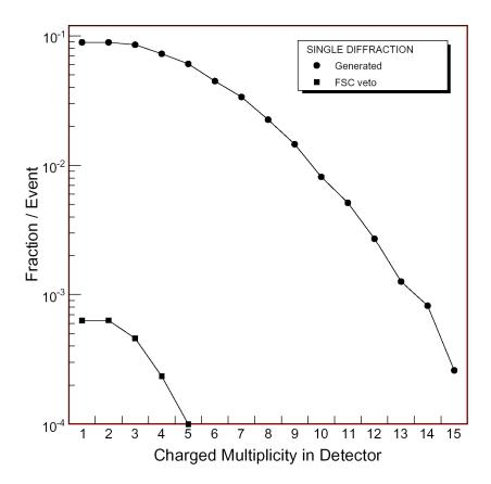
**Figure 3.** The probability per event for a given number of charged particles to be emitted within the spectrometer detector acceptance region is given by the upper curve (filled circles), the lower curve (filled squares) gives the acceptance with deployment of the FSCs.
