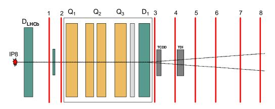
**Figure 1.** The layout of LHCb detectors at the LHC Interaction Point (IP8). The proposed Forward Shower Counters (FSCs) are shown as vertical lines (1 to 8). The locations of the dipole (D) and quadrupole (Q) magnet elements are shown as green (dark) and yellow (light) boxes.
