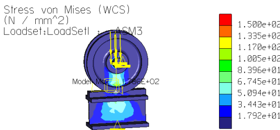
Figure 3.40: Von Mises stress for wheel-rail model in MPa
