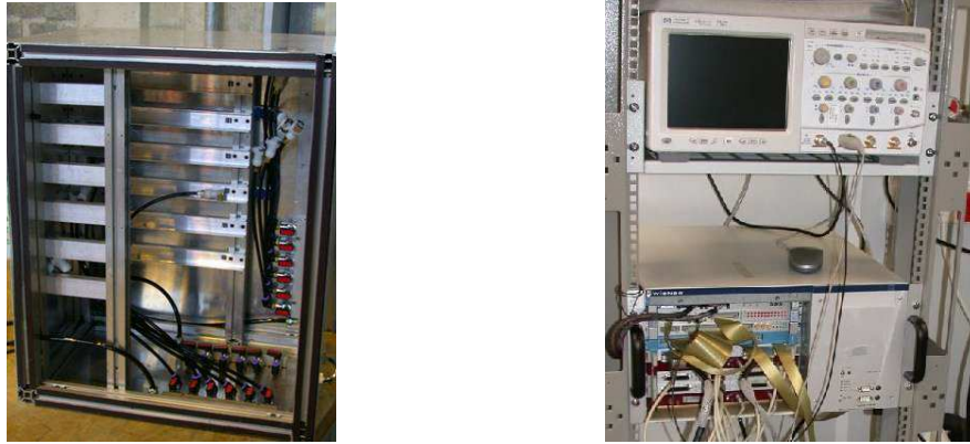
Figure 11: Electrical tests setup: the light-proof box (left) and the readout boards installed in the VME crate (right).
