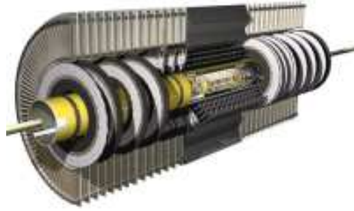
Figure 1: Layout of the ATLAS Inner Detector: it comprises the Transition Radiation Detector, the Semiconductor Tracker and the Pixel system from the outer to the inner radii, respectively.
