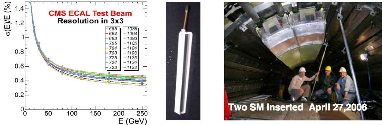
FIGURE 5. The CMS Electromagnetic Calorimeter (ECAL) (from left to right): the performance of 18 crystals in test beam; photo of an individual PbWO 4 crystal and the first two supermodules just after installation in April, 2006.
