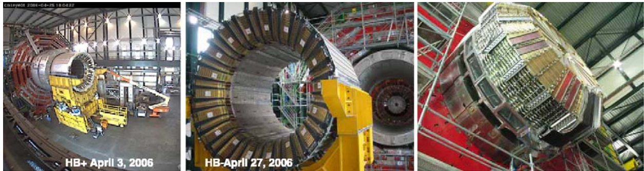
FIGURE 4. The CMS Hadron Calorimeter (HCAL): the two barrel sections (denoted HB+ and HB-) are shown during their installation in April, 2006. At right is one of the end caps (HF).
