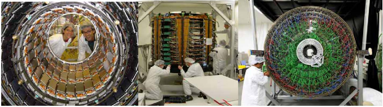
FIGURE 6. CMS silicon tracker subsystems in the Tracker Integration Facility at CERN are shown with some of the integration and testing personnel; from left to right the TIB, TEC and TOB.
