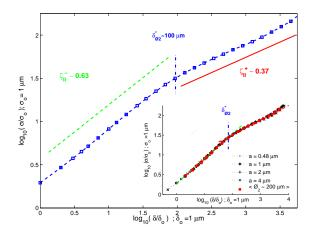
FIG. 2: Scaling behavior of the rms  $\sigma$  of the height fluctuations  $\Delta y(\delta)$  with two different roughness exponents  $\zeta_{\parallel}^- \sim 0.63$  and  $\zeta_{\parallel}^+ \sim 0.37$ , below and above the typical scale  $\delta^* \sim 100~\mu \mathrm{m}$  respectively. The inset shows that this scaling is independent of the image resolution a.
