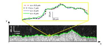
FIG. 1: A typical fracture (using glass beads of a diameter  $\varnothing_1 \sim 50 \mu m$  for roughening the samples) and a zoom of the crack front y(x) to emphasize the effect of the optical resolution given by the pixel size a.
