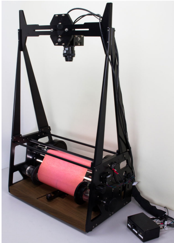
Figure 2: Stanford’s piano roll scanner built by Swope Design Solutions of San Francisco, California. A Welte T-100 piano roll is shown on the scanner.
