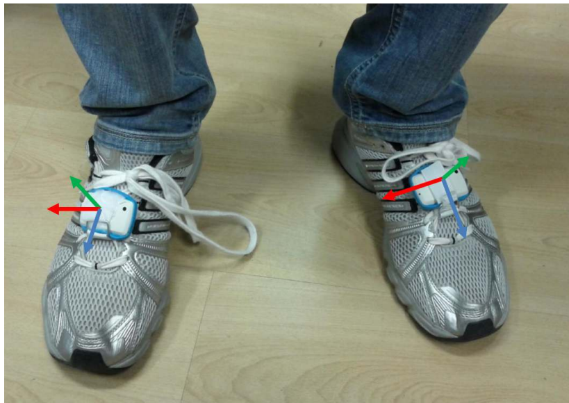
Figure 5.14: EXLs1 sensor nodes attached to the shoes. The body frames of the two sensors are aligned with x pointing to the user's right (in red in the figure), y forward (blue) and z up (green).
