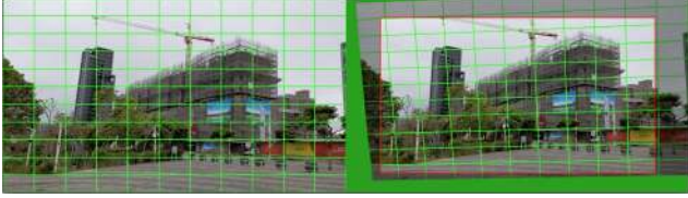
Figure 2: Grid-based frame warping. Left: the input frame with a regular 12x12 grid. Right: the warped frame with a virtual camera pose. The red bounding box shows the output frame after cropping. Note the rolling shutter distortion is also corrected (curved lines are straightened).
