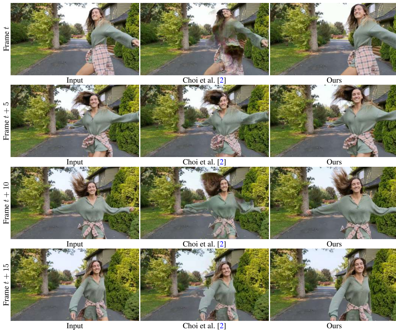
Figure 9: Visual comparisons with Choi et al. [2]. The method of Choi et al. [2] often generates ghosting and blurry results when the camera or object motion is large.
