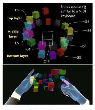
Figure 2: Top: the AR musical interface consists of three layers of coloured cubes and a cubic controller in the centre; touching each cube with a finger activates the corresponding tone. Bottom: an in-app view of the system in use.
