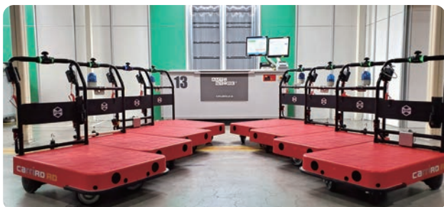
Logistics support robot CarriRo®. These self-driving carriages can read the sensors on workers’ uniforms and automatically follow them.
