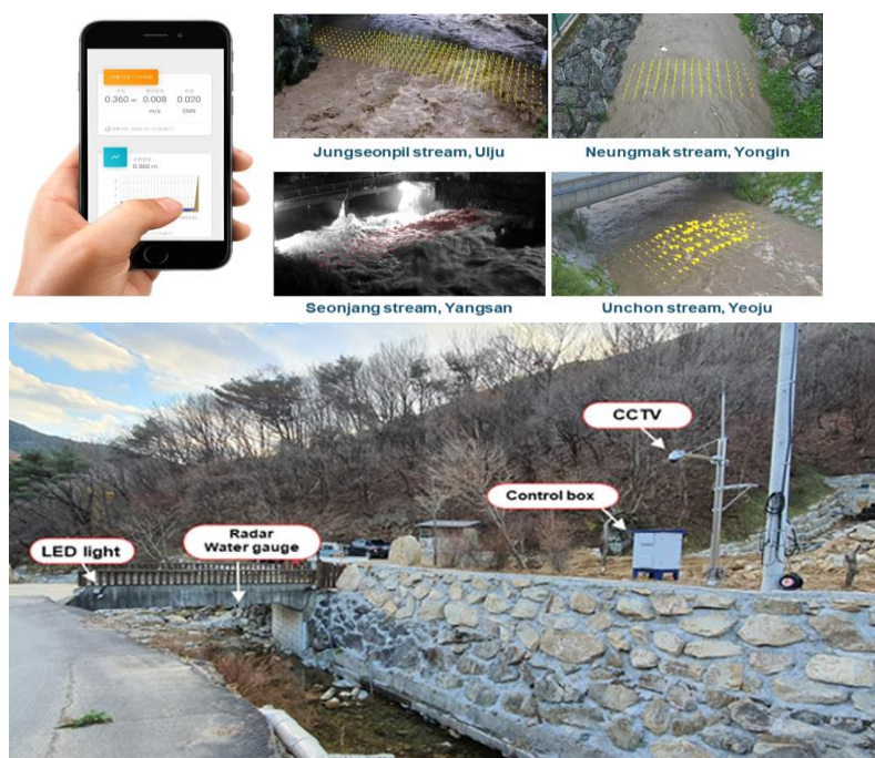
Figure 5.5. Example of CCTV based Automatic Discharge Measurement Technology
