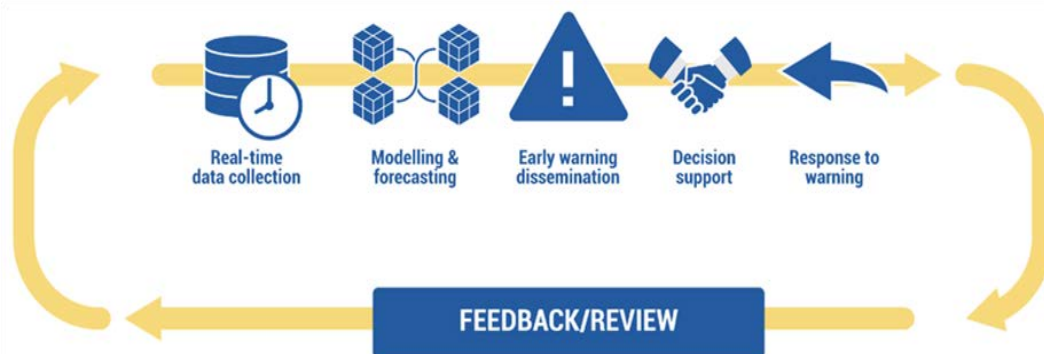
Figure 5.11. End-to-end early warning systems for flood forecasting
