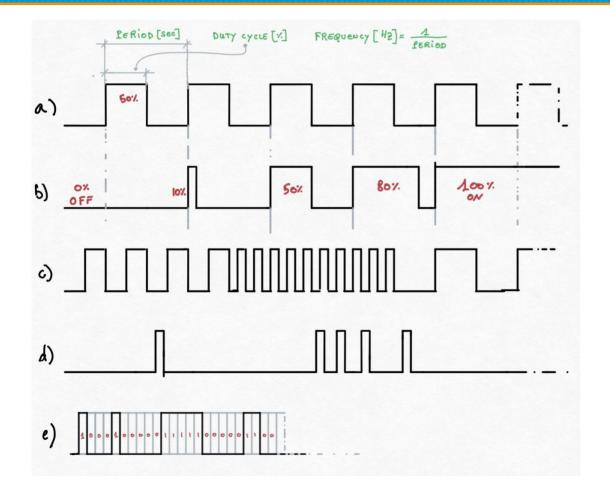
[a] Square wave, duty-cycle 50% [b] PWM. Width modulation. change the duty-cycle, e.g. dimming lights, DC motors speed, servo motor angle ... [c] Frequency modulation. e.q. sound, La (A) - 440 Hz. [d] Sparse pulses. e.g. Lovato power meter in S0, 1 pulse of 20ms per each 0.01kWh consumed. [e] Digital communication e.g. serial line, I2C ...
