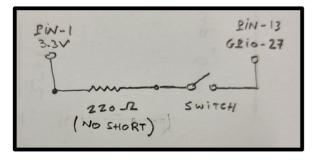
. tell the system that gpio27 is an input pin controlled by gpioirq----- /etc/gpio.conf -----# see gpioirq(4)gpio0 27 set in pd# first  $0x01 \rightarrow only gpio27$  controlledgpio0 attach gpioirq 27 0x01 0x01# second  $0x01 \rightarrow catch rising edges$
