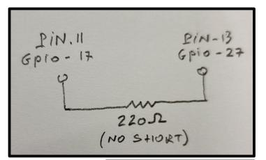
(\*) the resistor is not really necessary in this circuit because GPIO input pins have high impedance.
