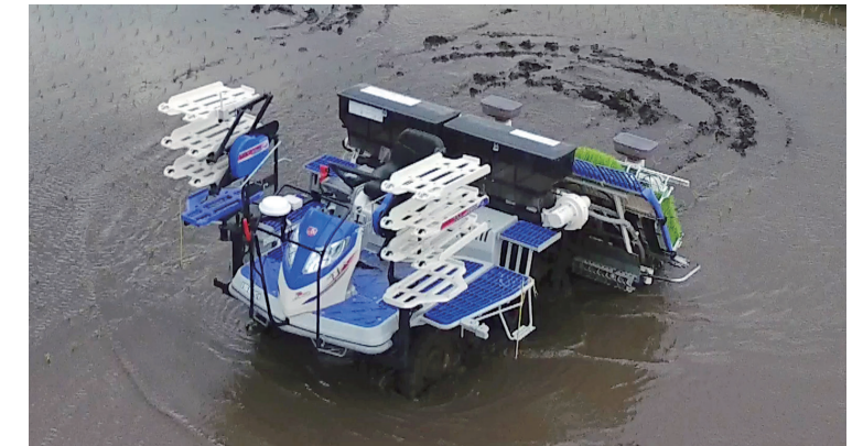
Autopilot rice transplanter developed by NARO through a national project "Cross-ministerial Strategic Innovation Promotion Program (SIP)" and is ready to go to market in February 2022
