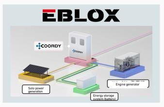
EBLOX is a stand-alone triple hybrid power system that makes the most out of renewable power sources by combining batteries with engine generators. We conducted demonstration studies in Japan and Turkey and are now planning full-scale sales.
