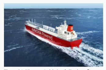
We completed the conceptual design of a Very Large Gas Carrier (VLGC) that can be converted from using LPG fuel to using ammonia fuel that does not emit CO<sub>2</sub>.
