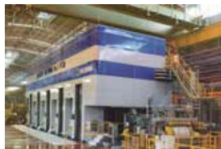
PL-TCM (Pickling line Tandem Cold Mill) for Posco-Vietnam
