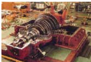
Steam Turbine Generator for Vina Kraft Paper (26MW)
