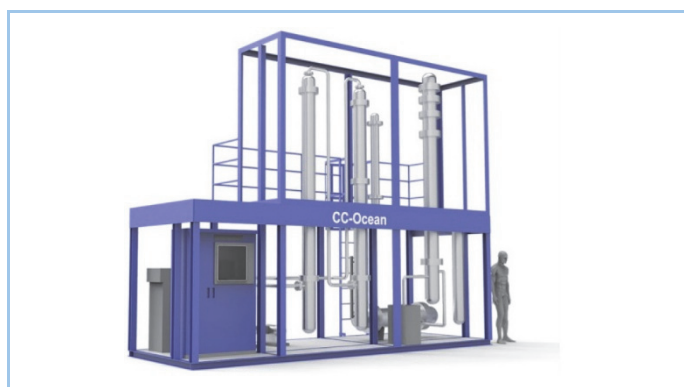
Figure 6 Illustration of installed small demonstration plant of onboard CO 2 capture system
