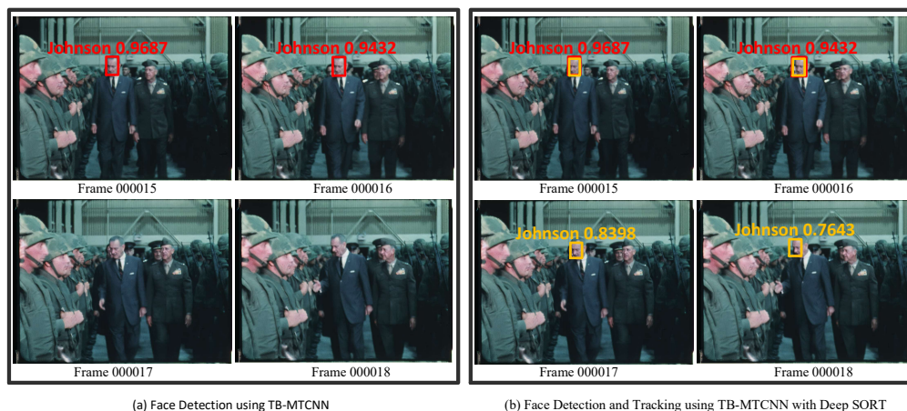
Figure 7. The Deep SORT method recovered the missed detections (the red boxes are faces detected using the TB-MTCNN detector, and the yellow boxes are faces recovered using Deep SORT).
