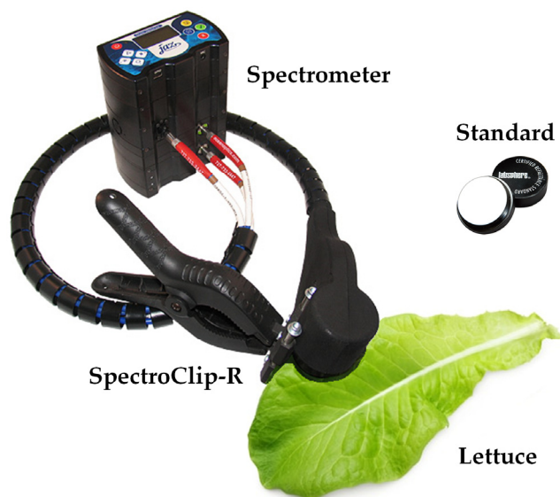
Figure 3. Hand-held spectrometer coupled to a clip probe for measuring spectral reflectance of the lettuce leaves.
