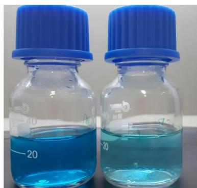
**Figure 4.** Residual baths from MB dyeing based on fabric untreated with  $\beta$ -CD (**left**) and MB dyeing based on fabric treated with  $\beta$ -CD (**right**).
