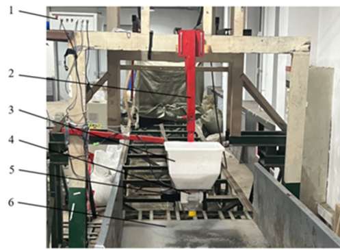
Figure 14. Bench test device. 1. Control box. 2. Fixed bracket. 3. Fertilizer tank. 4. Fertilizer distribution system. 5. Stepper motor. 6. Portable soil trench.
