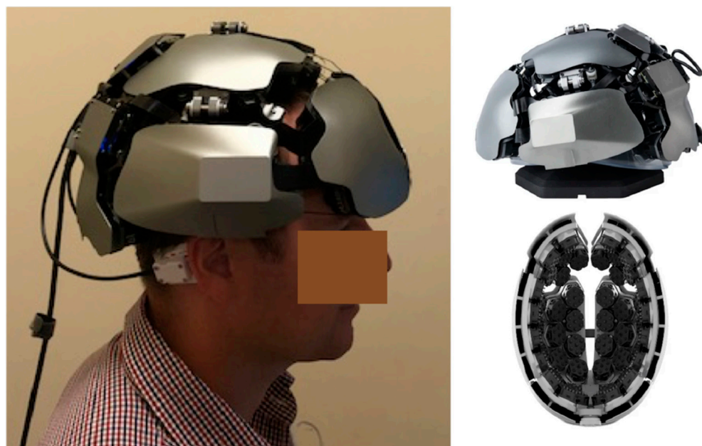
Figure 3. (Left): Side view of the Kernel Flow device (Kernel Inc. (Los Angeles, CA, USA)) for noninvasive optical brain imaging. (Right): Outer and inner views of the Kernel Flow headset [12,15] demonstrating the wearable form.
