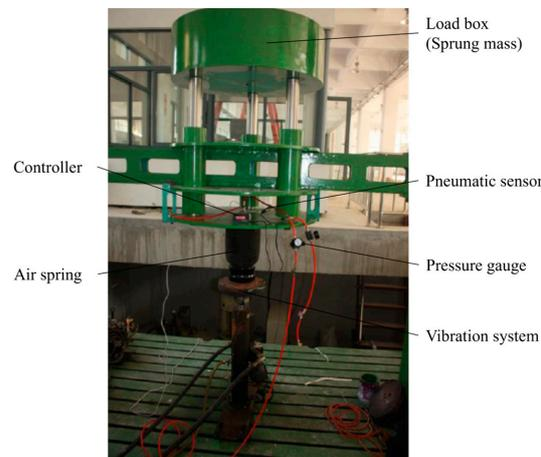
Figure 10. Experimental device of suspension.
