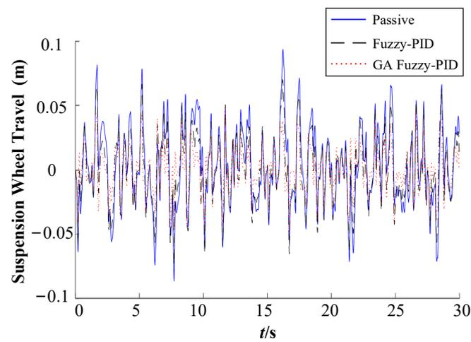
Figure 15. Simulation of suspension wheel travel.
