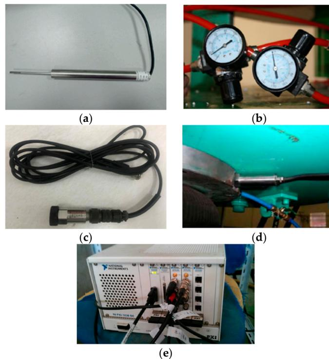
Figure 11. Experimental device of suspension. (a) Displacement sensor. (b) The barometer. (c) Acceleration sensor. (d) Pressure transducer. (e) NI data acquisition instrument.
