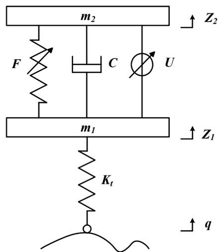
Figure 1. 1/4 Two-Degree-of-Freedom Model of The Vehicle.
