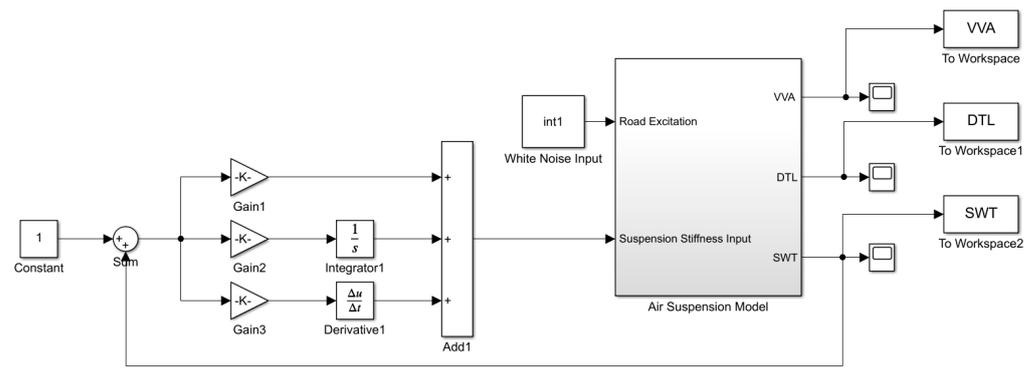
Figure 4. PID Simulation System of Air Suspension.
