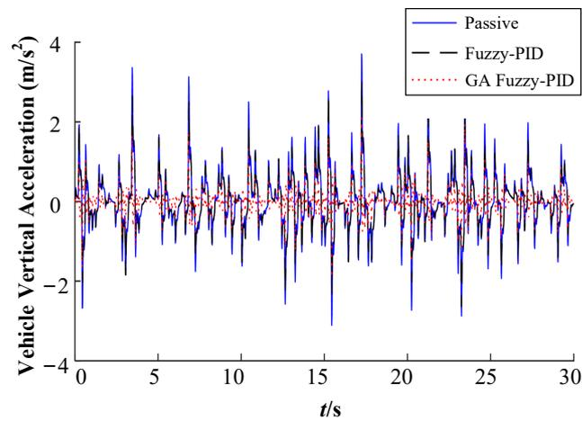
Figure 14. Simulation of vehicle vertical acceleration.
