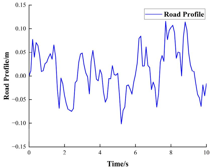
Figure 3. Time domain curve of B road surface.
