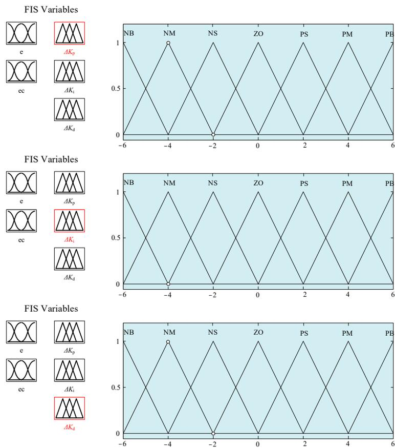
Figure 7. Output membership function curve.
