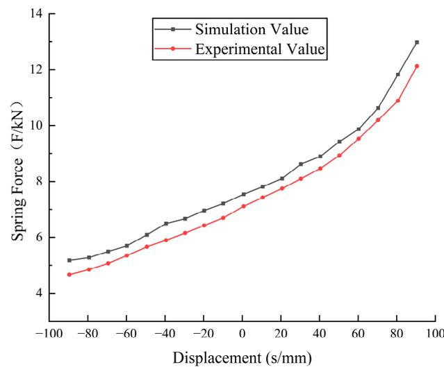
Figure 13. Comparison of response curves between simulation results and test results.
