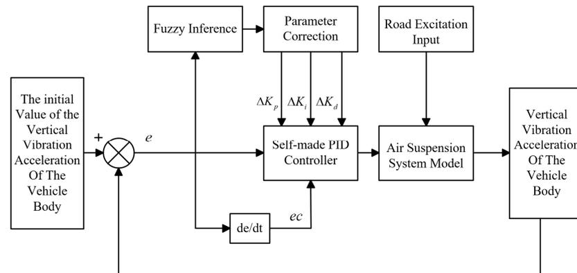
Figure 5. Schematic Diagram of Fuzzy PID Controller.
