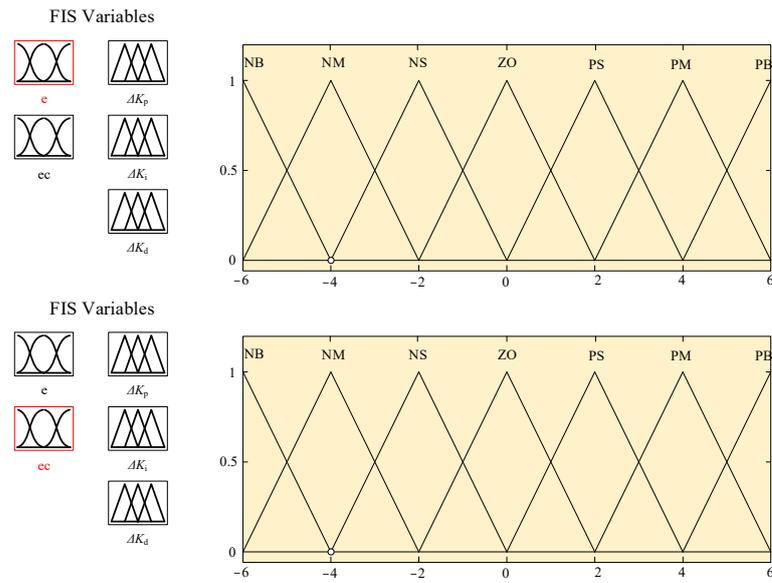
Figure 6. Input membership function curve.
