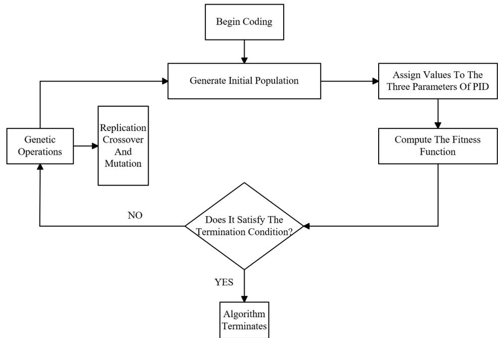
**Figure 8.** The Basic Program of Genetic Algorithm.
