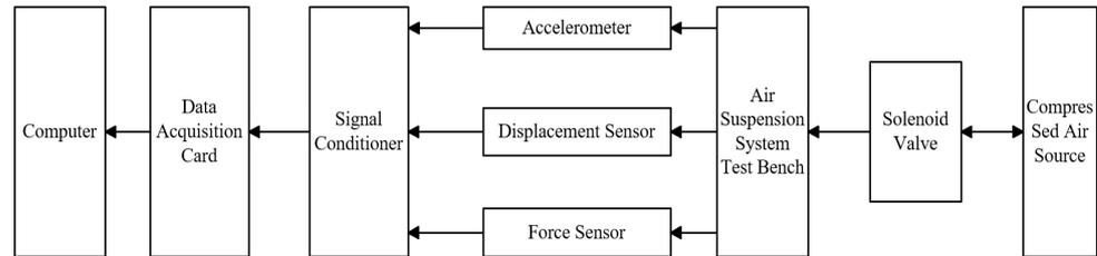
Figure 12. Block diagram of air suspension test bed.
