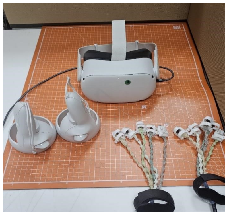
Figure 4. Experimental setup with Oculus Quest 2 and vibrotactile glove components.
