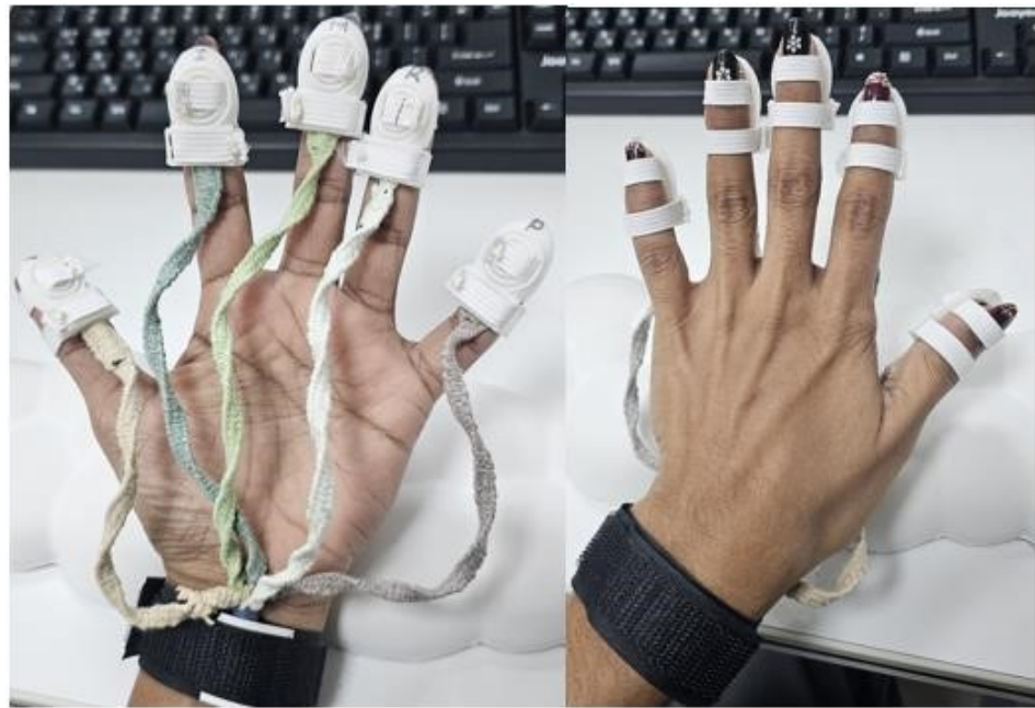
Figure 2. Design of custom 3D-printed fingertip holders for ERM motors.
