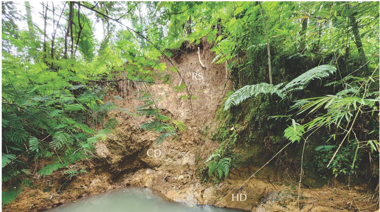
**Figure 3.** Typical outcrop of brown residual soil and yellowish brown completely and highly decomposed tuffs. RS: residual soil; CD: completely decomposed tuff; HD: highly decomposed tuff.
