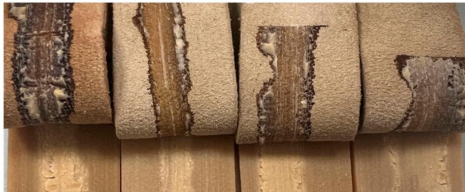
**Figure 12.** Appearance of samples after T-peel test. From left to right: HMPUR-REF, LIGNOC-2.5%, LIGNOC-5%, and LIGNOC-7.5%.
