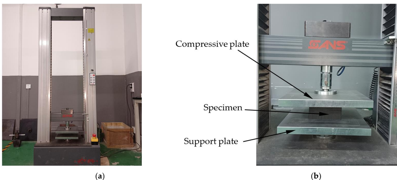
Figure 2. Testing machine used for compression of EVA foam specimen: (a) Universal material testing machine; (b) Specimen in compression.
