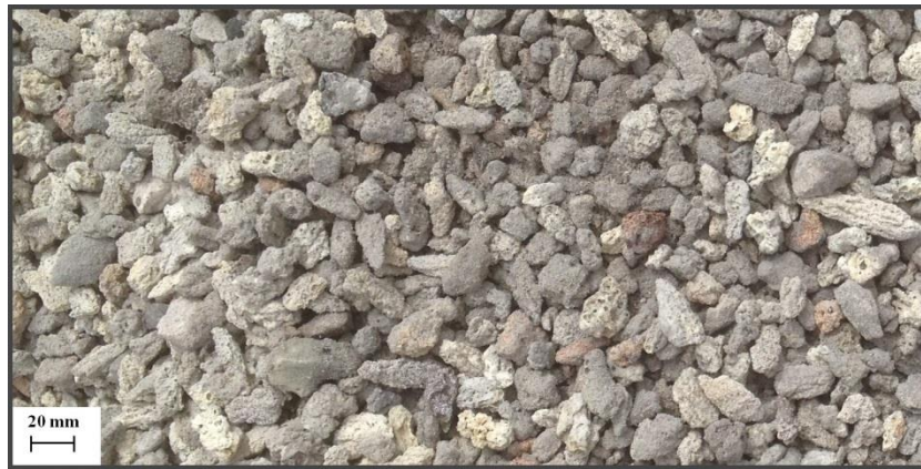
Figure 5. The bottom ash particles employed in this application.
