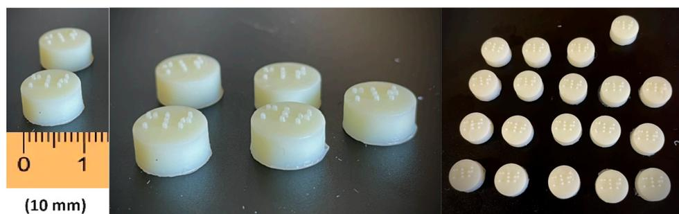
**Figure 2.** The MLT 3D-printed tablets with Braille patterns.**Table 2.** Printing parameters set on the LCD 3D printer.
