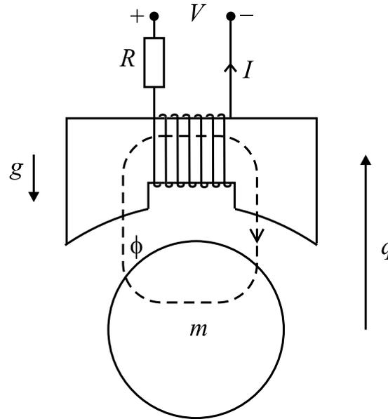
$$\begin{bmatrix} \dot{q} \\ \dot{p} \\ \dot{\phi} \end{bmatrix} = \begin{bmatrix} 0 & 1 & 0 \\ -1 & 0 & 0 \\ 0 & 0 & -\frac{1}{R} \end{bmatrix} \begin{bmatrix} \frac{\partial H}{\partial q} \\ \frac{\partial H}{\partial p} \\ \frac{\partial H}{\partial \phi} \end{bmatrix} + \begin{bmatrix} 0 \\ 0 \\ 1 \end{bmatrix} V, \quad I = \frac{\partial H}{\partial \phi}(q, p, \phi)$$
