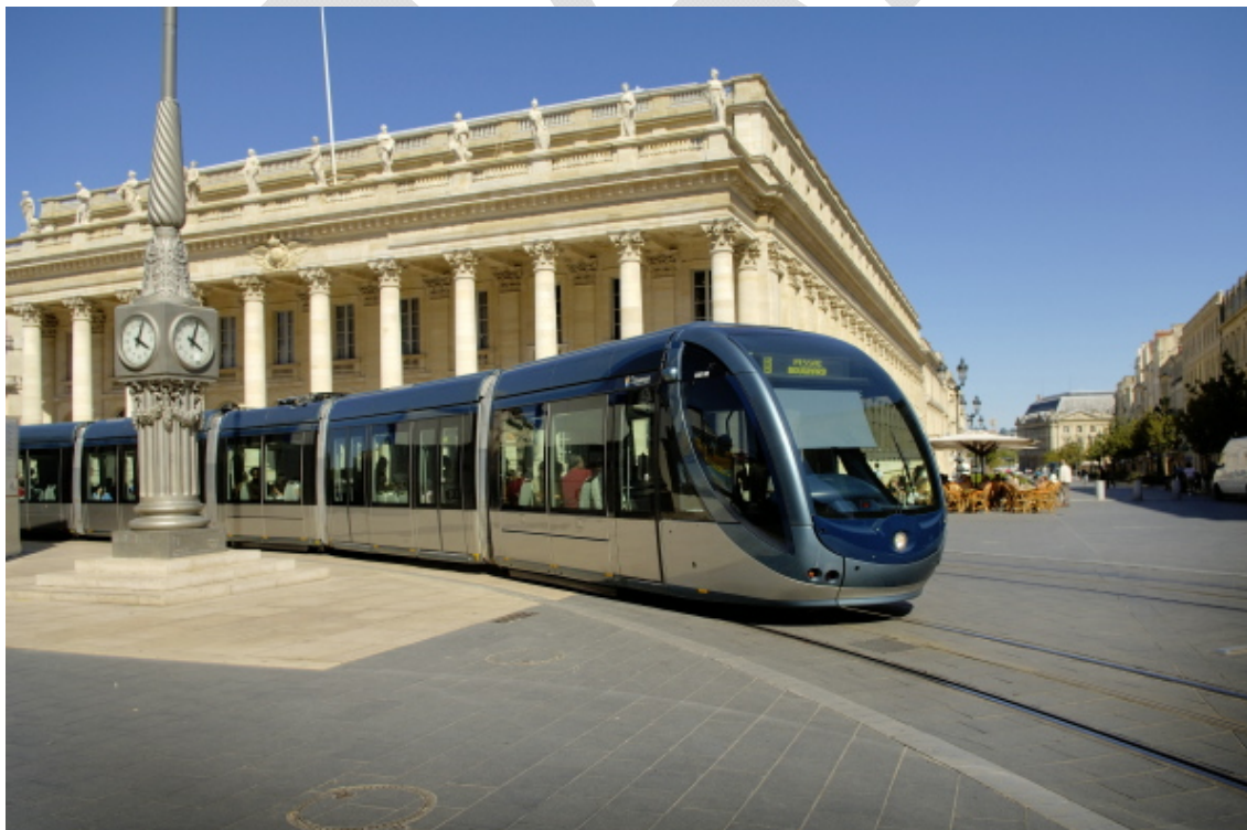
Figure 4-27: Embedded Power Rail (Citadis, by Alstom)
