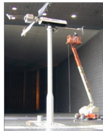
(b) Full scale NREL Phase VI wind turbine blade.
