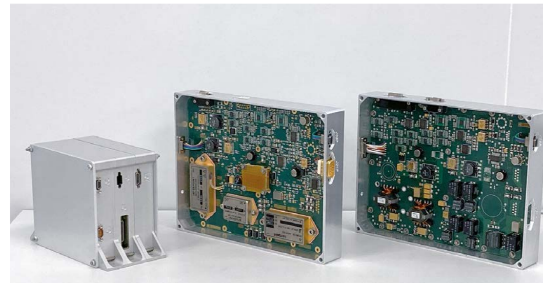
Comet Interceptor Elegant Breadboard Models electronics for EnVisS (left), MANiaC (center), CoCa (right)
