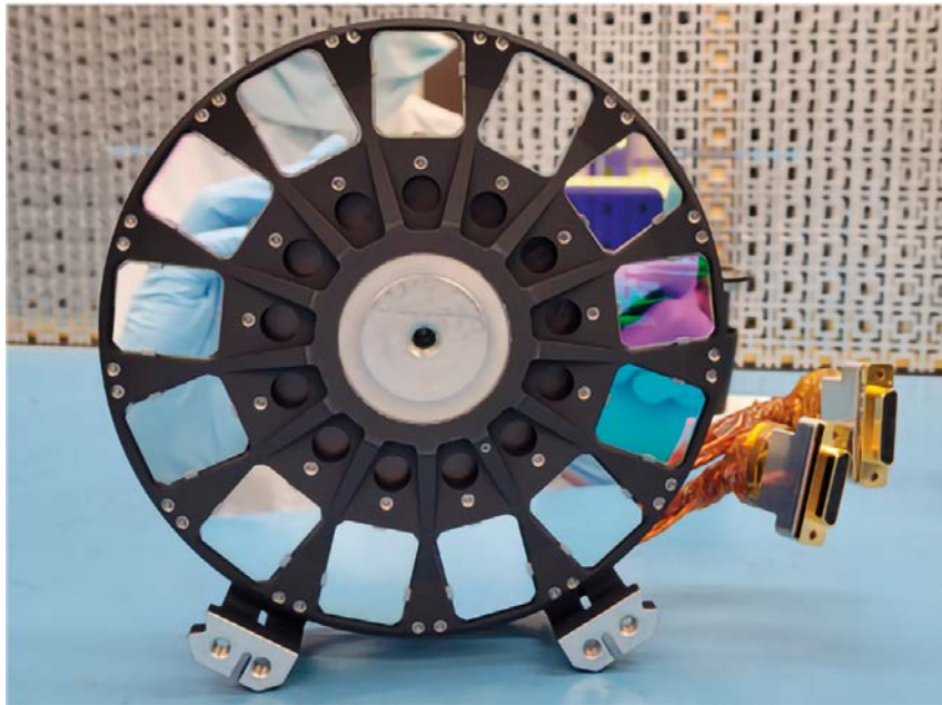
Flight Models of the JANUS instrument for the JUICE Mission: Filter Wheel
