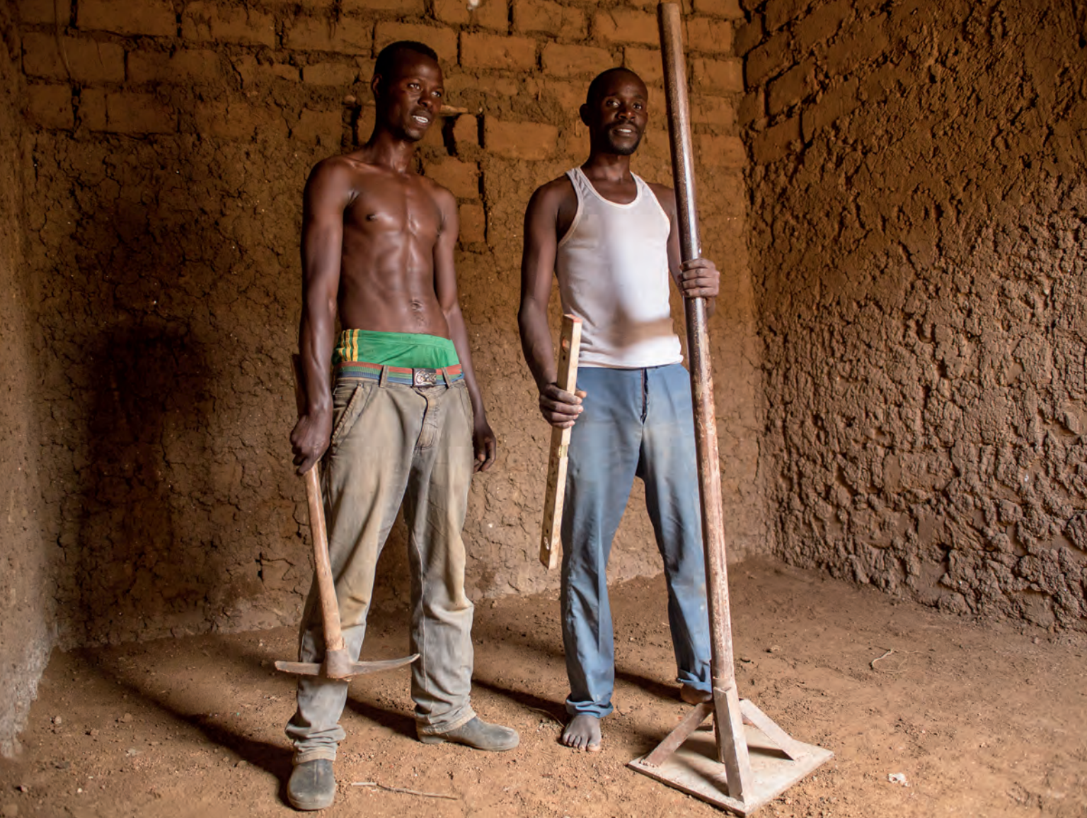
TOOLS OF THE TRADE Masons use tampers and levels to ensure that the floors are well-compacted and sloped for drainage.
