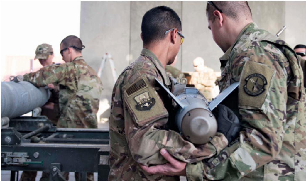
Munitions flight crew carry the tail kit of a GBU-54, a 500-pound Laser Joint Direct Attack Munition. (U.S. Air Force photo)
