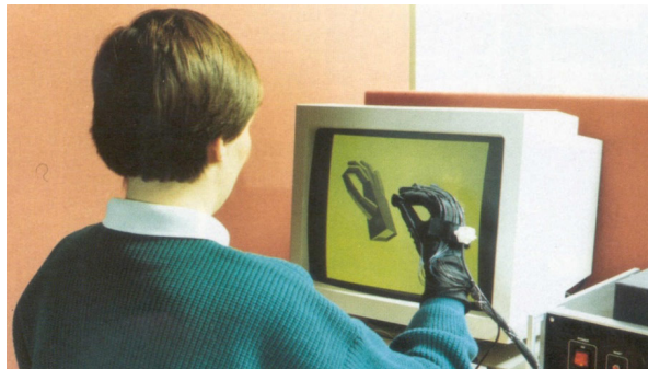
The DataGlove, created by VPL Research. See database entry.
