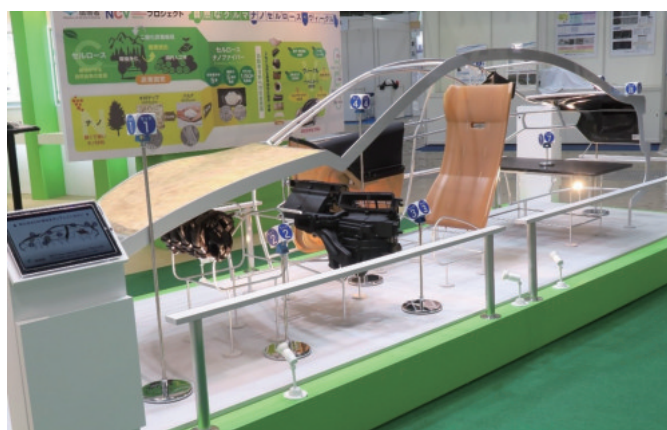
Photo 1 Trial manufacture of automobile parts using CNF composite material
