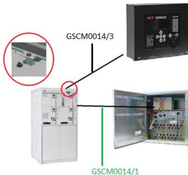
Figure 2 - Principle diagram of connections between Switchgears-RGDM-UP in according to GSCM004, GSCM005
