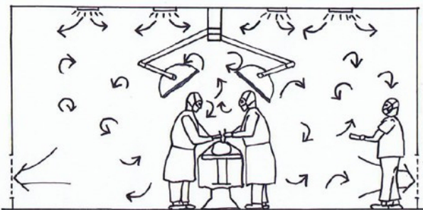
Figure 3: Mixed air ventilation with an air quality that is the same everywhere.
