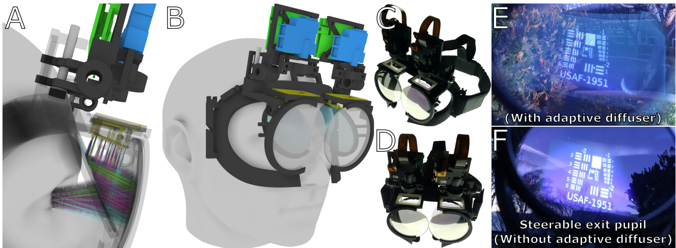
Figure 1: (A) A three dimensional rendering of our proposed near eye display's optical layout that is based on projection light engines with moving lenses colored in sky blue, three dimensionally printed application-adaptive optical diffusers colored in yellow, beam-splitters colored in dark blue, partially reflective beam combiners colored in white, and electronics colored in green. (B) A three-dimensional rendering showing our wearable near eye display design. (C-D) Actual photographs showing our printed wearable prototype from different perspectives, (E-F) Actual photographs showing how a single eye of an user observe high resolution augmented content displayed with our prototype at a sunset scenery. Top photograph is taken when an application-adaptive optical diffuser is used. Bottom photograph is taken without application-adaptive optical components leading to a steerable exit pupil. Both cases has the ability to steer the image by moving lenses of a projection light engine, promising a design candidate to future foveated near eye displays.
