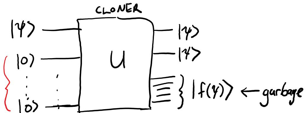
$$\text{so } U(|\psi\rangle \otimes \underbrace{|00\dots 0\rangle}_{n-1}) = |\psi\rangle \otimes |\psi\rangle \otimes \underbrace{|f(\psi)\rangle}_{2^{n-1}\text{-dimensional}}$$
