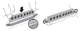
Using firm, even pressure, push UDIMM/CUDIMM into slot until clips snap into place. Do not assist clips.
