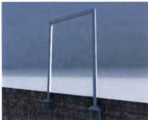
Step 4: Finishing linking bridge at top of towers
