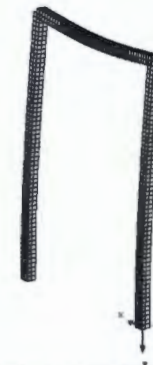
Deflection due to wind in y-direction (amplified)
