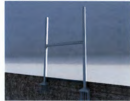
Step 3: Lifting of linking bridge
