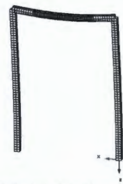
Deflection due to wind in x-direction (amplified)
