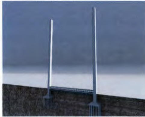
Step 2: Tower shafts and assembling of linking bridge on ground level.
