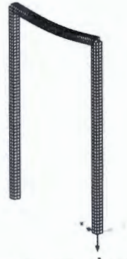
Deflection due to dead load (amplified)
