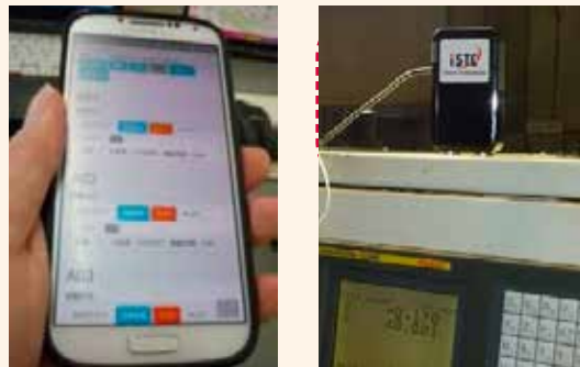
A computer terminal for handling remote monitoring of the manufacturing line (left) and a transmitter in the plant (right)
