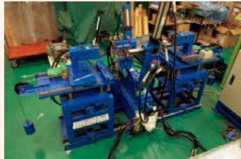
The specially-ordered coil-winding robot that boosted the company's productivity
