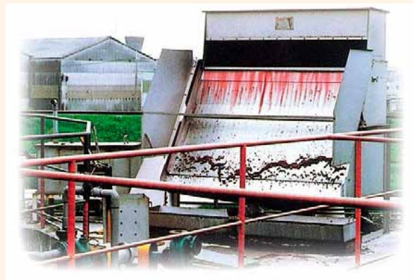
Toyo Screen Kogyo's Ultra-TN Screen (A diagonally-positioned apparatus using a wedge wire screen for the separation of solids and liquids)
