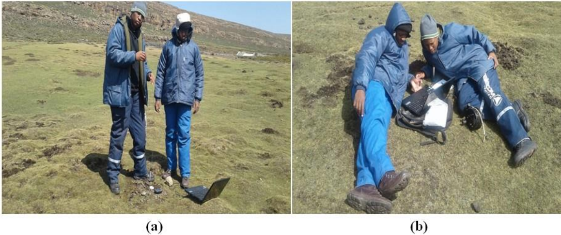
Fig. 9: Shows retrieving data logger from the piezometer (a) and data downloading (b)
