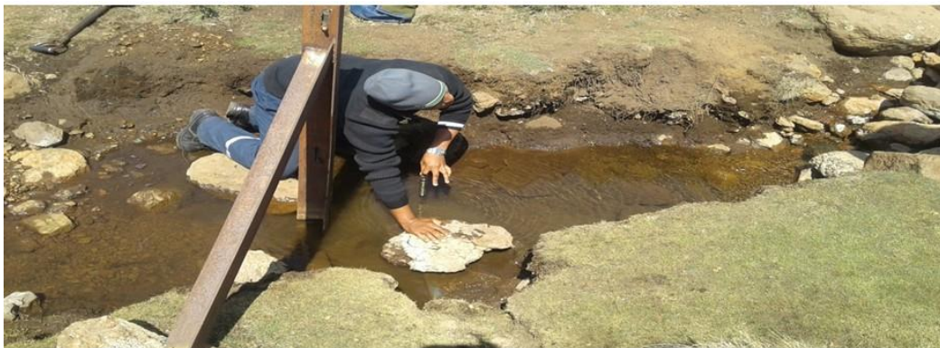
Pic. 11: Retrieving data logger from the draw box
