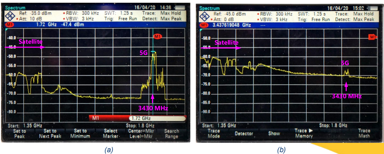
Figure 7 Spectrum plots at the Type-B LNB output: (a) before and (b) after tightening the BPF-LNB interface screws.
